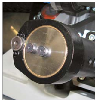
▲ Option - Bending heads that can be moved off center enable the use of the most diverse tool concepts
