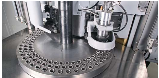
▼ Grinding table and spring length measuring device (in-process)
