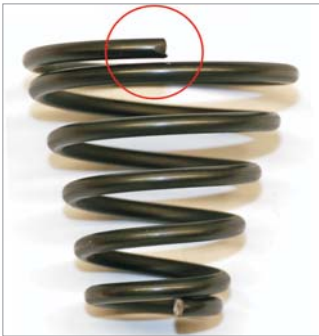
▲ Conical spring produced without PTP coiling finger
