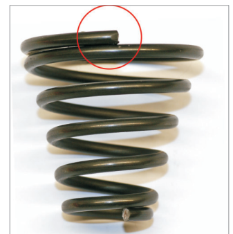
▲ Conical spring produced with PTP coiling finger
