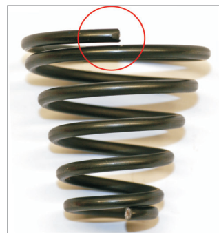
▲ Conical spring produced without PTP coiling finger
