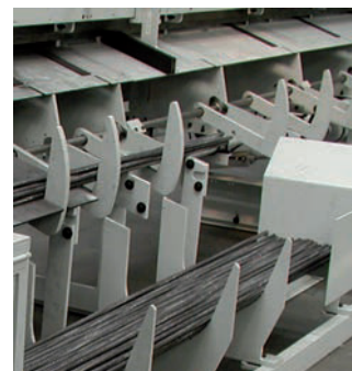
▲ Stop of tilting station and rod-end alignment
