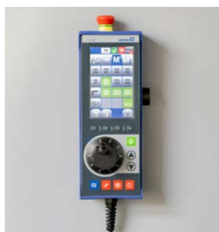
▲ Hand-held operating device with Touch Screen
