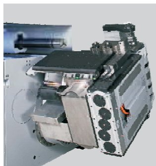
▲ Heavy-duty bending head with open clamping
