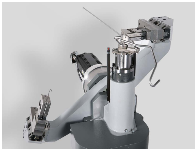
▼ Bending head TWISTER 2 12-RL
