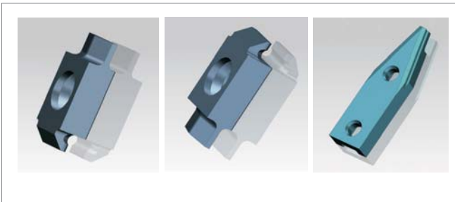
▲ Plate for bending and erecting loops, winding plate
