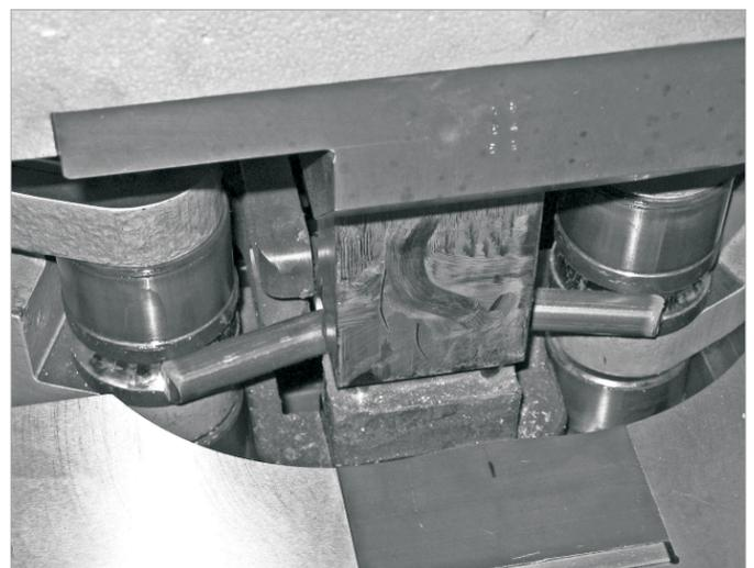
▲ KER-bending lever with rollers
