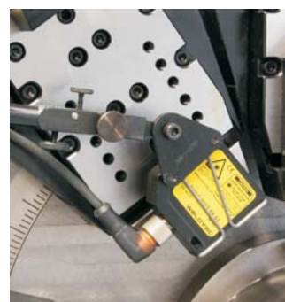
▲ Ejection control with laser
