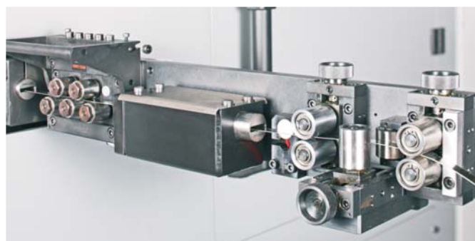
▲ Straightener with Strip material guide and end-of-strip-material control
