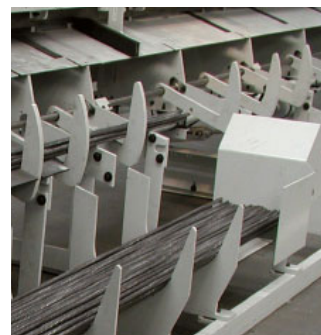
▲ Stop of tilting station and rod-end alignment
